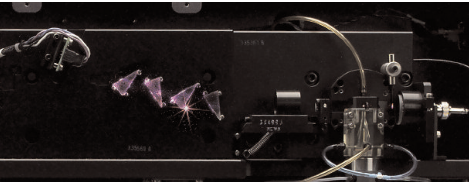
Figure 3 Beam-shaping optics and flow cell.
