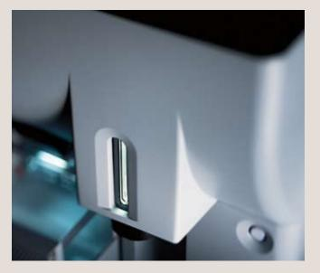
The BD FACSAria<sup>™</sup> cell sorter sets a new standard for highperformance flow cytometry. Based on an entirely new design in instrumentation, the BD FACSAria instrument is the first benchtop sorter that incorporates a fixed-alignment cuvette flow cell that can detect up to 13 colors, for a total of 15 parameters. The cuvette flow cell allows for up to three aircooled or solid state lasers at 488 nm, 633 nm, and 405 nm.
