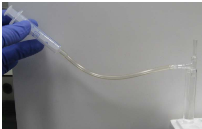
Figure 3.9. Flexible tubing attached to both Syringe and Side Arm of Nebulizer
