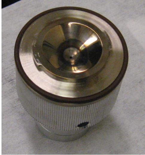
Figure 3.5. The sampler attached to the Cones Removal and Installation Tool
