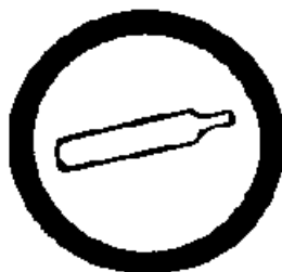
Figure 2-8 Compressed Gas Hazard
