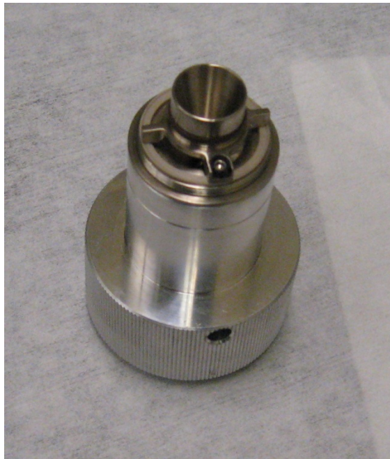
Figure 3.6. Skimmer-reducer Assembly attached to the Cones Removal and Installation Tool
