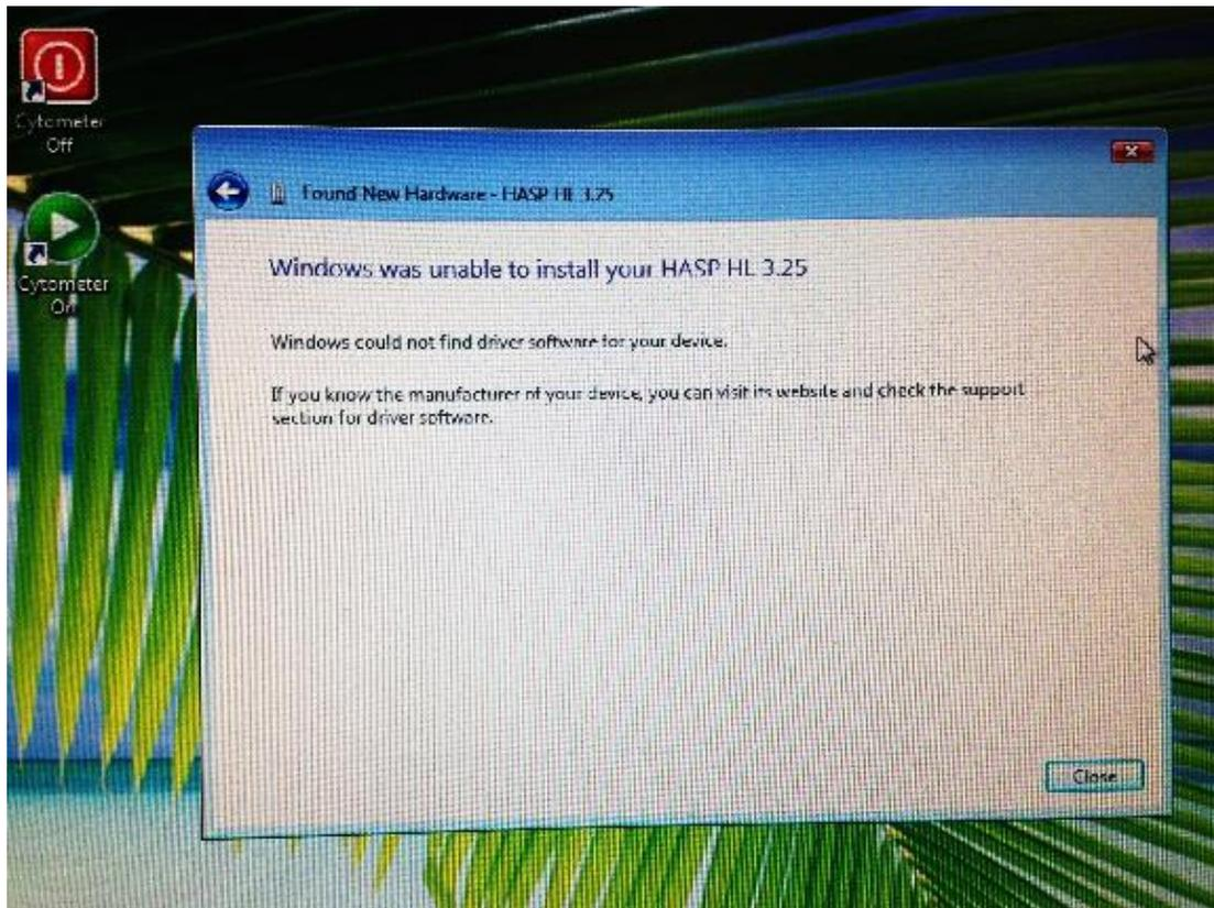
5.3.2. Those error message are generated by Windows that is capable to detect correctly the HASP key BUT not able to install the HASP Driver.
